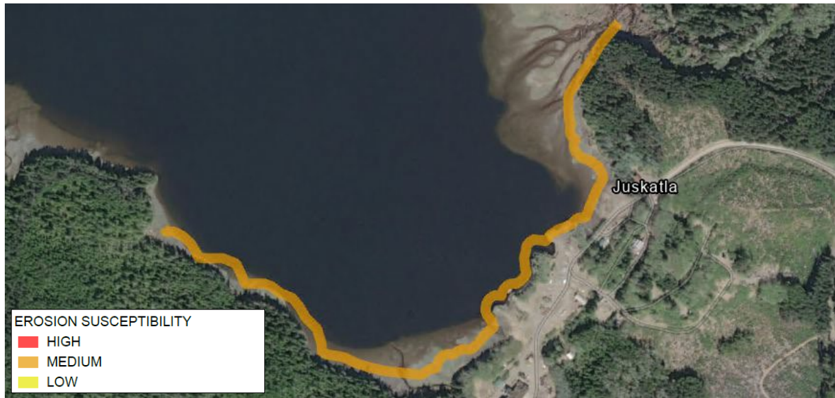
Figure 3-1. Map of erosion susceptibility for the Juskatla portion of the study area.
