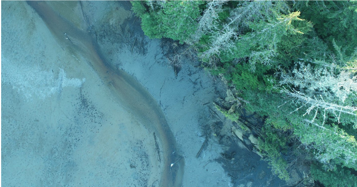
Figure 3-5. Aerial image of the northeastern shoreline in Juskatla. Mature vegetation growing to the typical high tide line indicates a generally stable shore, and shallow waters offshore offer some protection from waves.
