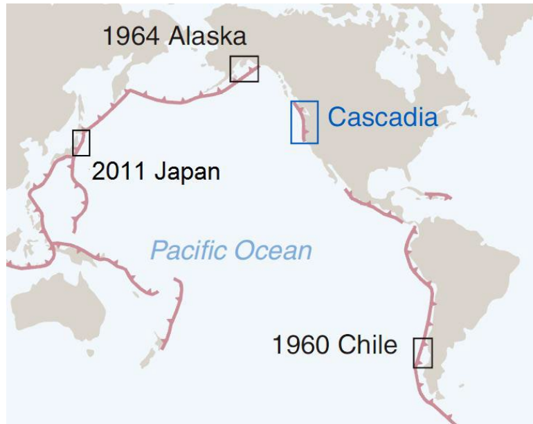
Figure 3-8. Subduction zones around the Pacific Ocean and locations of several major tsunamigenic earthquakes (adapted from Atwater et al., 2005).
