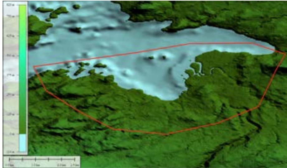
Figure 4. Polygon representing the area in which CADEM was lowered by 3m in the Juskatla area to ensure consistency with NHC Juskatla survey.
