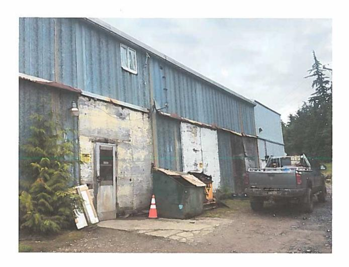
Going to get rid of the sliding door and tracking to the left of the garbage bin and will be replacing with a wall. Will be getting a new door to replace the aluminum one. Will be replacing the other bay doors and tracking as well. The doors to the far right I will be extending to 18 feet high.
